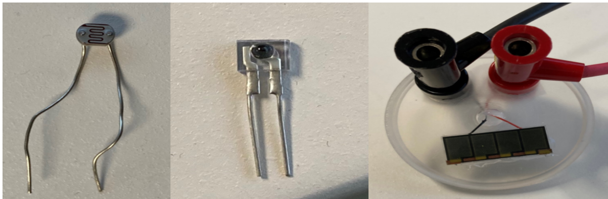
Figure 9: Photodetectors (from left to right) - A Photoresistor, Phototransistor, and Solar Cell
