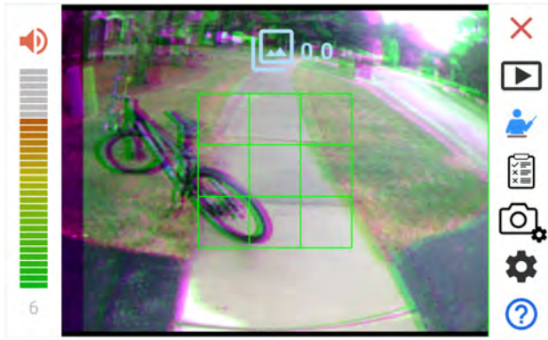
Fig. 2. The graphical user interface of 3DEye in the stereo disparity mode, displayed on the touch screen of a smart phone. Left RGB image: overlaid luminance as green; right RGB image: overlaid luminance as purple. The disparity value is heard through the earphone, and marked also visually by the left vertical bar.
