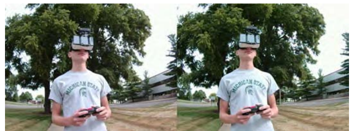
Fig. 1. Stereo images of a user operating a 3D system. The system has two video cameras, a mobile phone, a 3D viewing goggle and a game controller.
