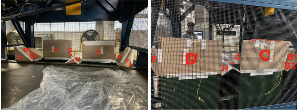
Figure 28: Photographs of the prototyped chute shields labeled by the components in the CAD.
