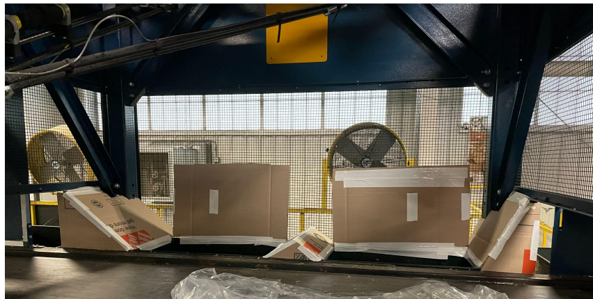
Figure 6: Prototyped cardboard chute diverters and lids.
