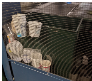
Figure 4: Photograph of recyclables lodged between the chute and cage.
