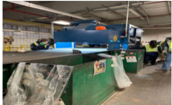
Figure 2: Items entering the robots vision system to then be sorted
